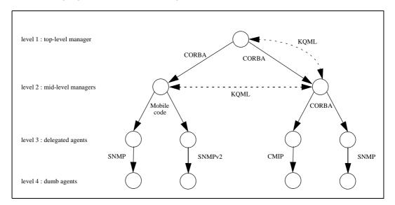
Figure 5 : Distributed network management: the integration model
