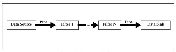
Figure 5-1: Processing Pipeline
