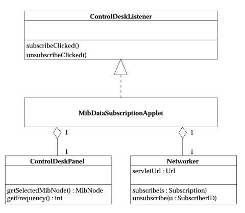
Figure 6.4: Classes of the MIB data subscription applet involved in the subscription system
