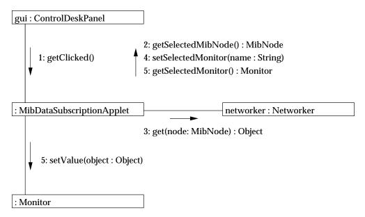
Figure 6.7: Get operation in the MIB data subscription applet
