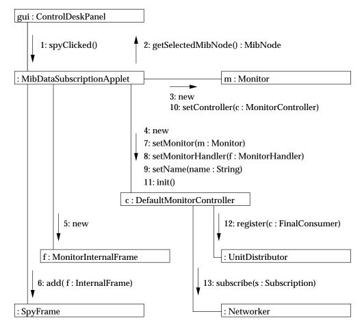
Figure 6.10: Adding a spy to the spy frame of the MIB data subscription applet
