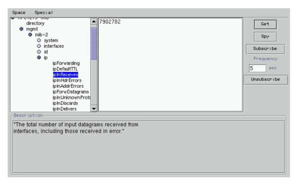
Figure 5.2: The MIB data subscription applet GUI
