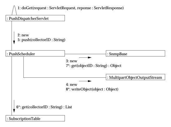
Figure 6.17: Push scheduling in the push dispatcher servlet.
