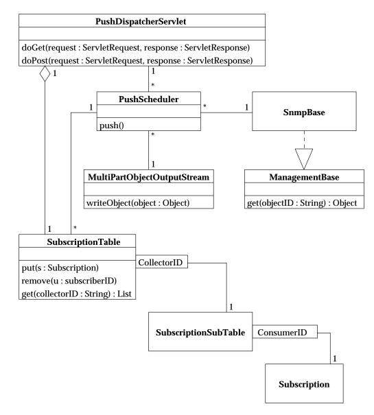
Figure 6.16: Classes of the push dispatcher servlet
