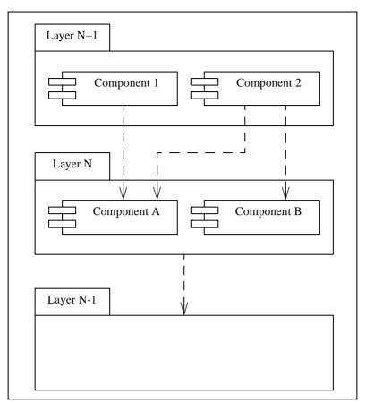
Fig. 4: Shielded and Unshielded Layers
